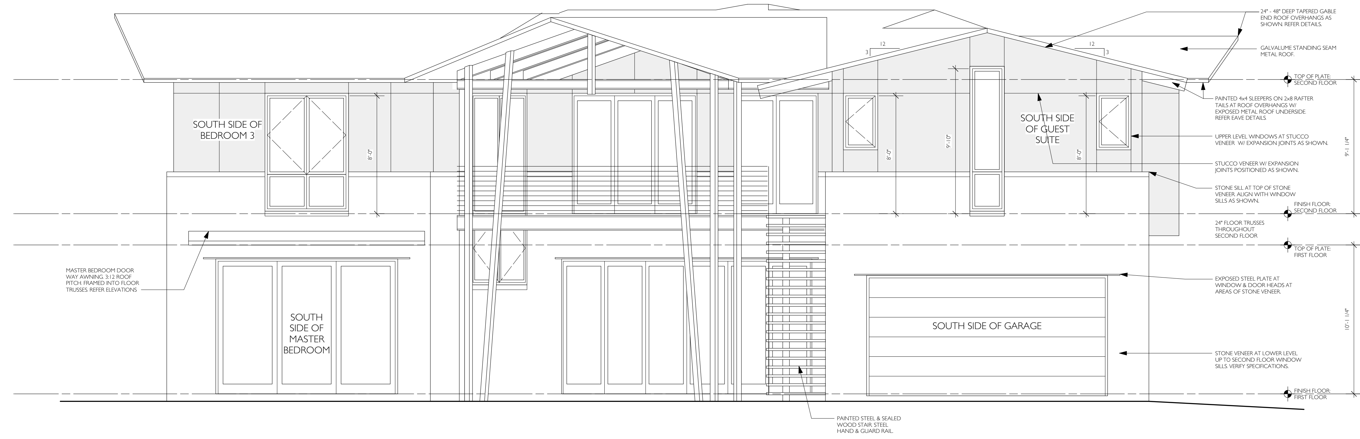
2 MASTER BEDROOM, BEDROOM, GARAGE & GUEST SUITE SOUTH ELEVATION SCALE: 1/4" = 1'-0"
